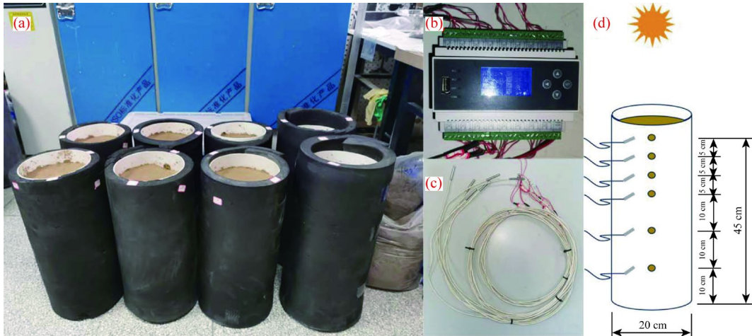
Fig. 1 Apparatus of the evaporation experiment. (a), soil column; (b), multichannel recorder; (c), temperature probe; (d), schematic of the placement of temperature probes.
